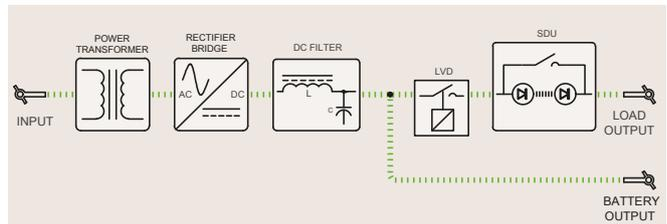
The power transformer adjusts the network voltage close to the DC charging voltage. Thyristor bridge that is connected to the secondary windings of the power transformer provides AC/DC voltage conversion and DC voltage adjustment. Output filters are used to keep the OUTPUT voltage stable and low ripple.
