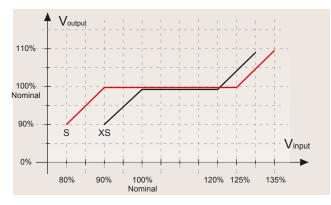
There are 2 options for output voltage tolerance in ELC Line Conditioner&Saver as +/-1% and +/-2%. The output voltage tolerance is related to the thyristor configuration used and affects the manufacturing cost.
