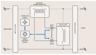
ELC Line Conditioner&Saver works on the principle of injecting voltage to the load supply voltage by the help of transformer connected in series between the network and load.
