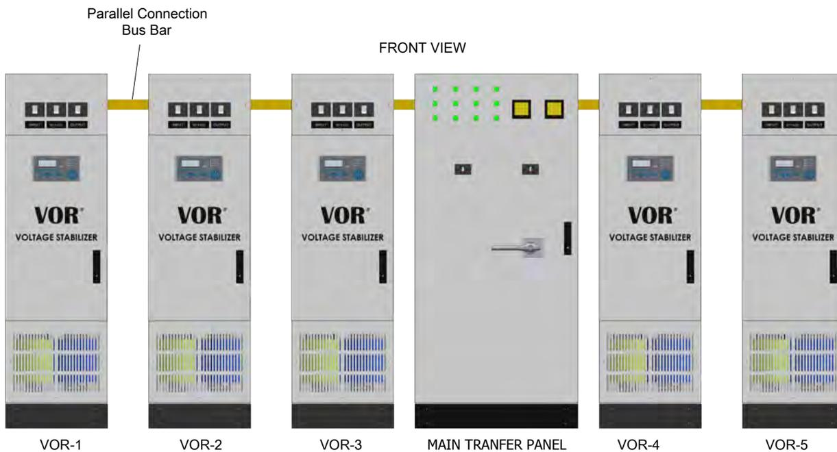
Figure - 9: Parallel Connection Application - II
