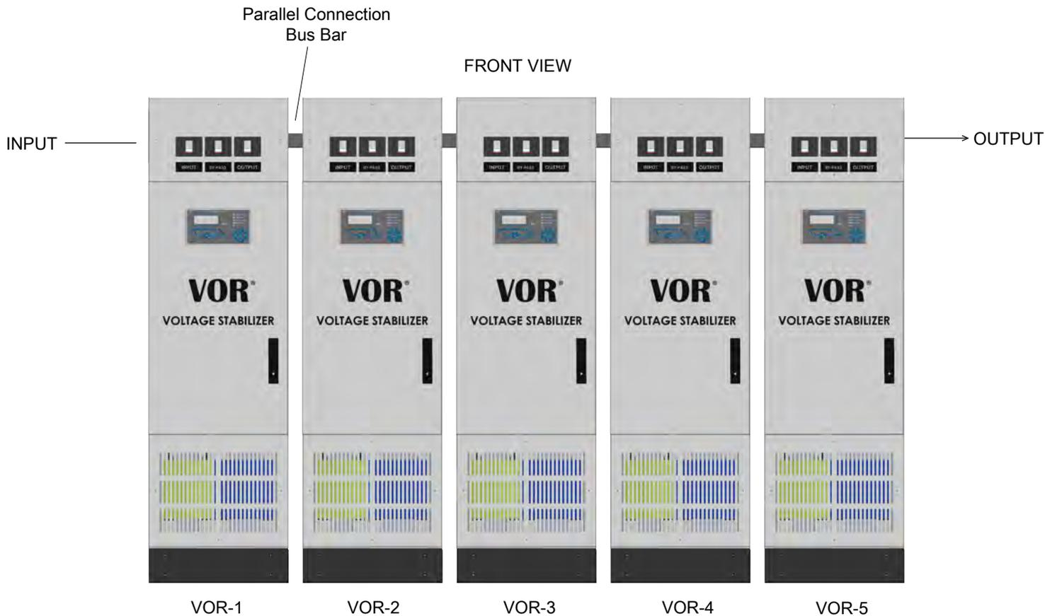
Figure - 9: Parallel Connection Application - I
