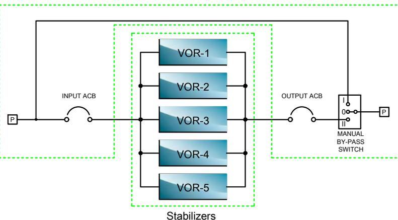
Figure - 1: Parallel redundant voltage management solution.
