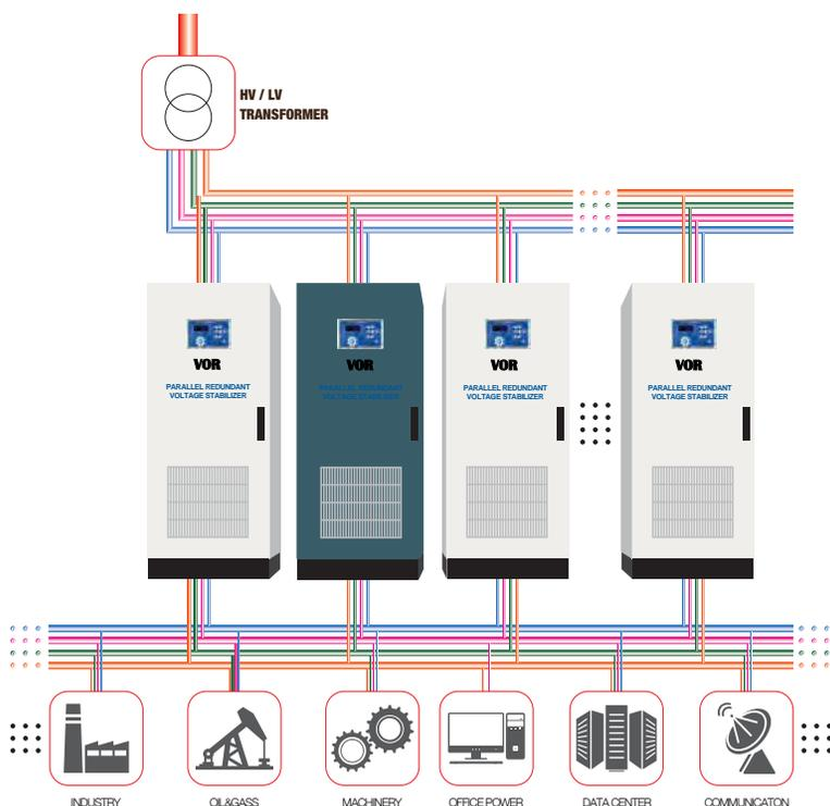
Figure - 1: Parallel redundant voltage management solution.
