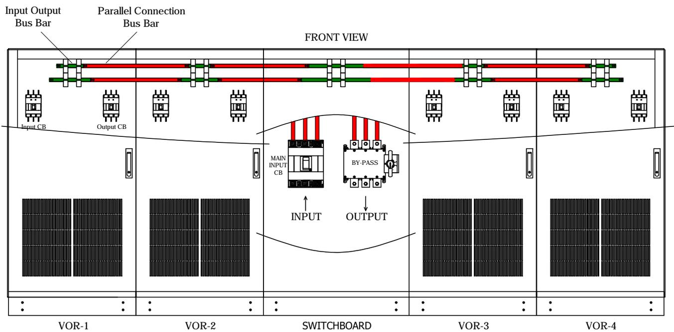
Figure - 9: Parallel Connection Application - II
