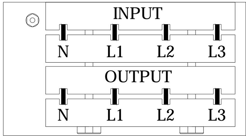
Note: The above busbar measures are the S model device. Busbar measures change in other models.
