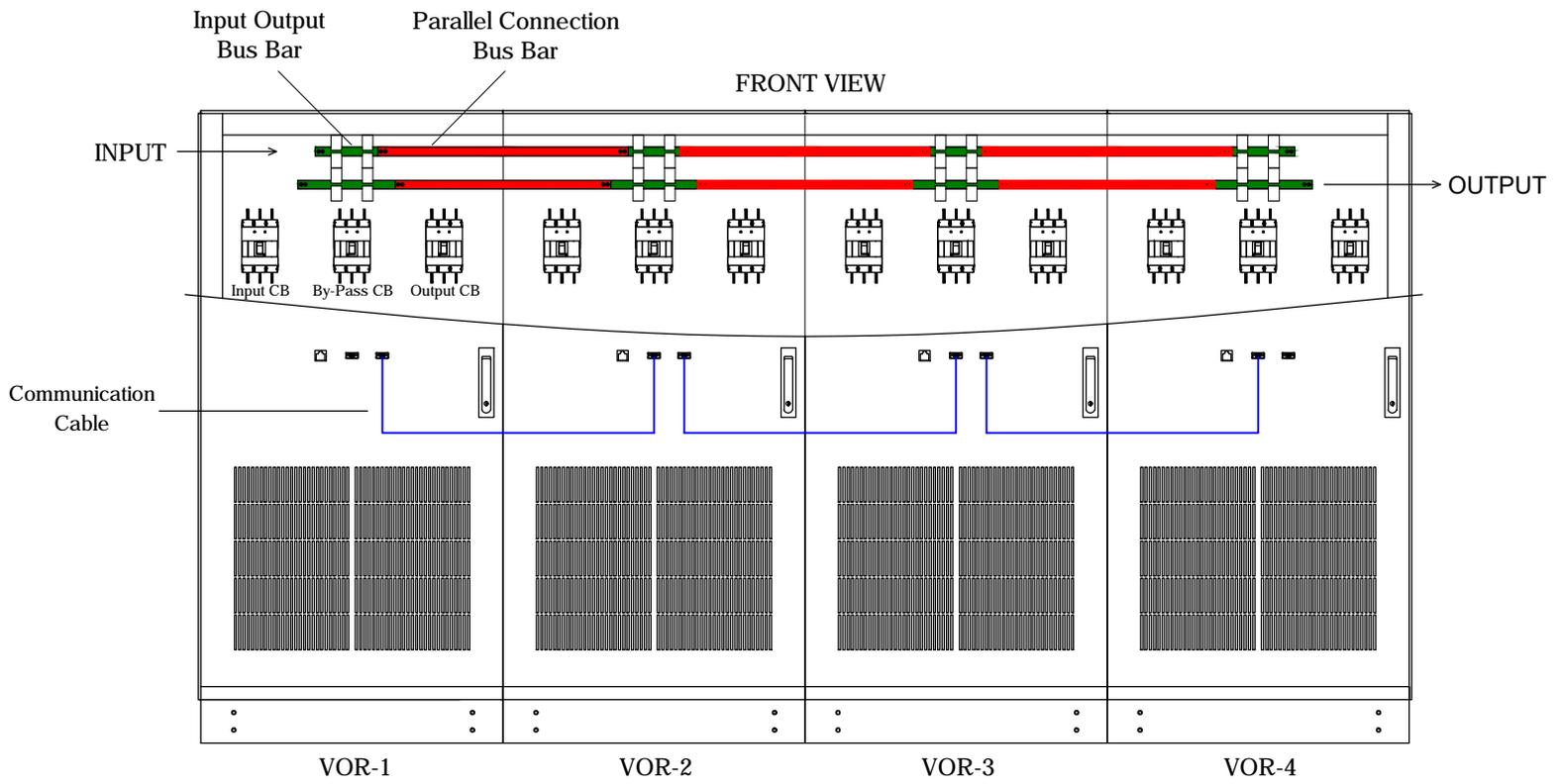
Figure - 9: Parallel Connection Application - I
